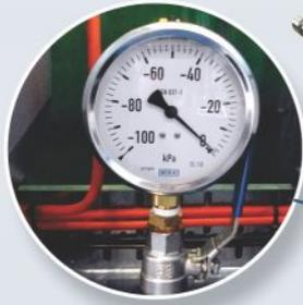
Liquid filled gauge with isolating valve for easy replacement
