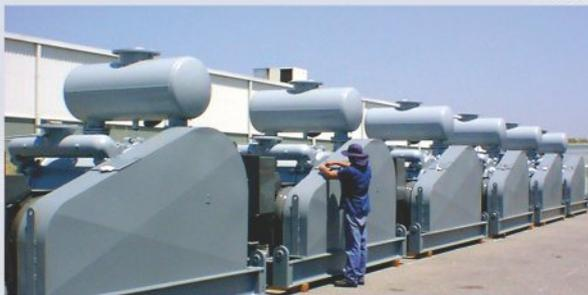
315 kW, 4,000 Nm<sup>3</sup>/h Pumps for Alumina Seed Filters – West Australia
